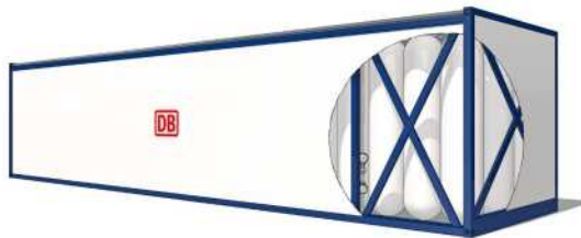
Figure 1: DB Cargo's multi-element gas container (MEGC) is used for transporting pure, gaseous hydrogen by rail.
