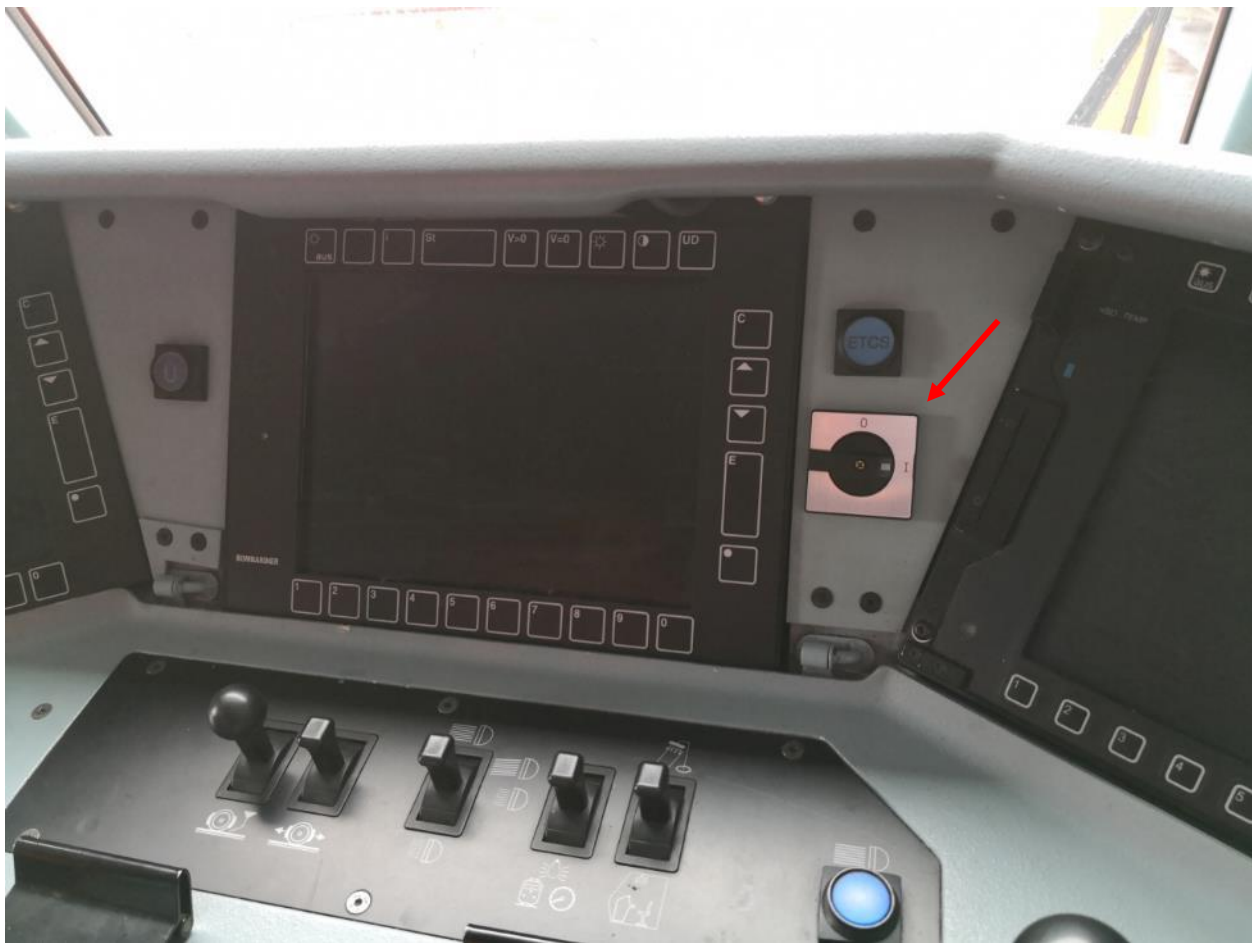
Figure 8: Power supply switch for ATO system in the driver's table
