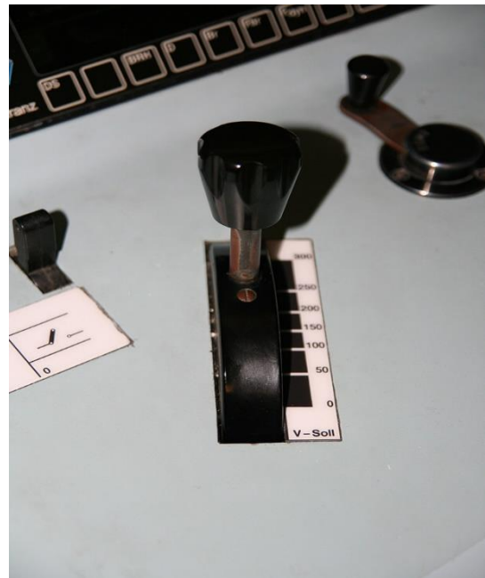
Figure 16: AFB Vsoll adjuster of ICE 1
