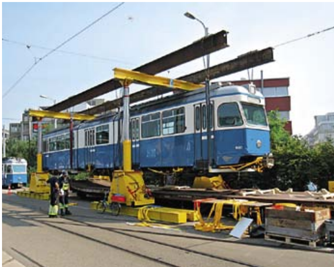
Zürich: A special timber structure and additional straps were used to secure the 20-metre long trams.
