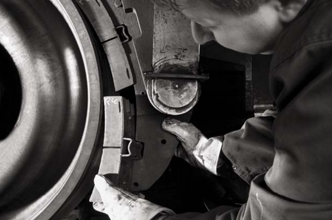
Whisper brakes: these innovative brake blocks are made of a composite material which does not roughen the wheels and therefore keeps noise to a minimum.
