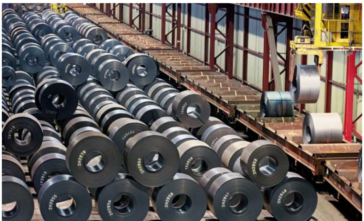
Loading hot strip coils onto Sah-series flatbed wagons in ThyssenKrupp Steel’s Dortmund plant
