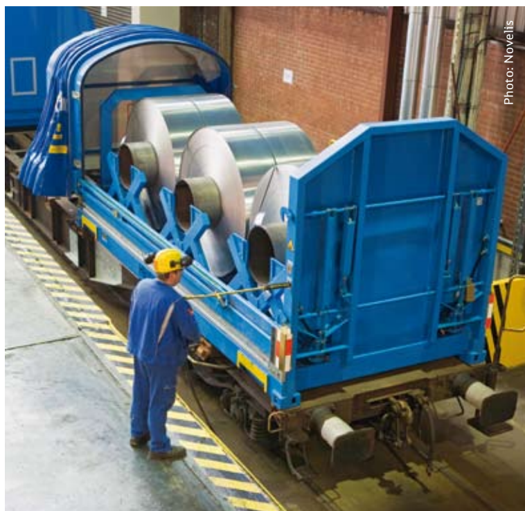
The containers were especially developed for rail transport and are opened using a special compressed air technique
