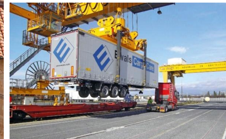
TRANSHIPMENT: gantry cranes lift heavy mega-trailers onto the wagons.
